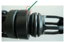
2. Rotate the element and slide it on the center tube of the housing cover afterwards.
